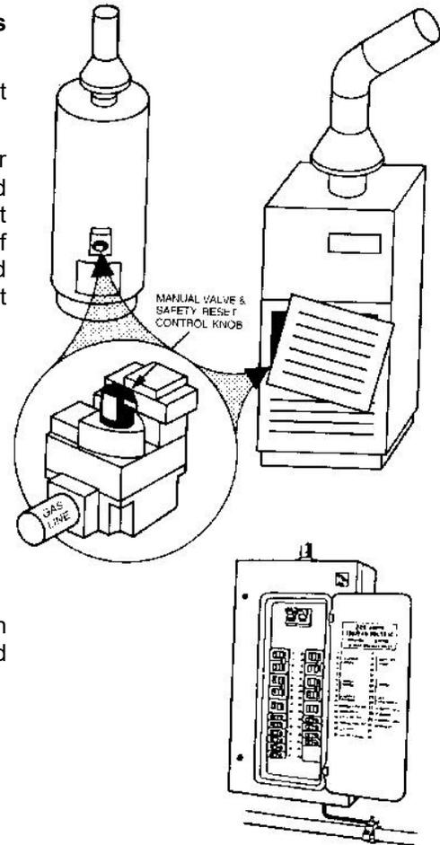
**ELECTRIC CIRCUIT BREAKERS AND FUSES** can malfunction when water and silt get inside. Discard ALL circuit breakers and fuses that have been submerged.
